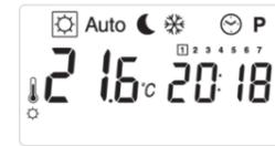
A press on (OK) key allows the displaying of comfort setpoint temperature.
