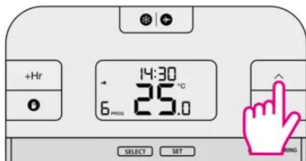
Using  $\wedge$  or  $\vee$  buttons set new setpoint temperature.
